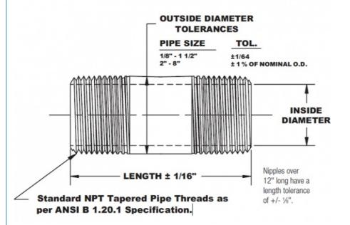
Pipe Pipe Length Size O.D. Close Nipple Lengths(Inches) in in in 1/8 0.405 <sup>3</sup>/4 4 41/2 5 51/2 6 7 8 9 10 11 12 1<sup>1</sup>/2 2 2<sup>1</sup>/2 3 3<sup>1</sup>/2 41/2 5 51/2 6 7 8 9 10 11 12 <sup>1</sup>/4 0.54 7/8  $1^{1}/2$ 2  $2^{1}/2$ 3  $3^{1}/2$ 4
