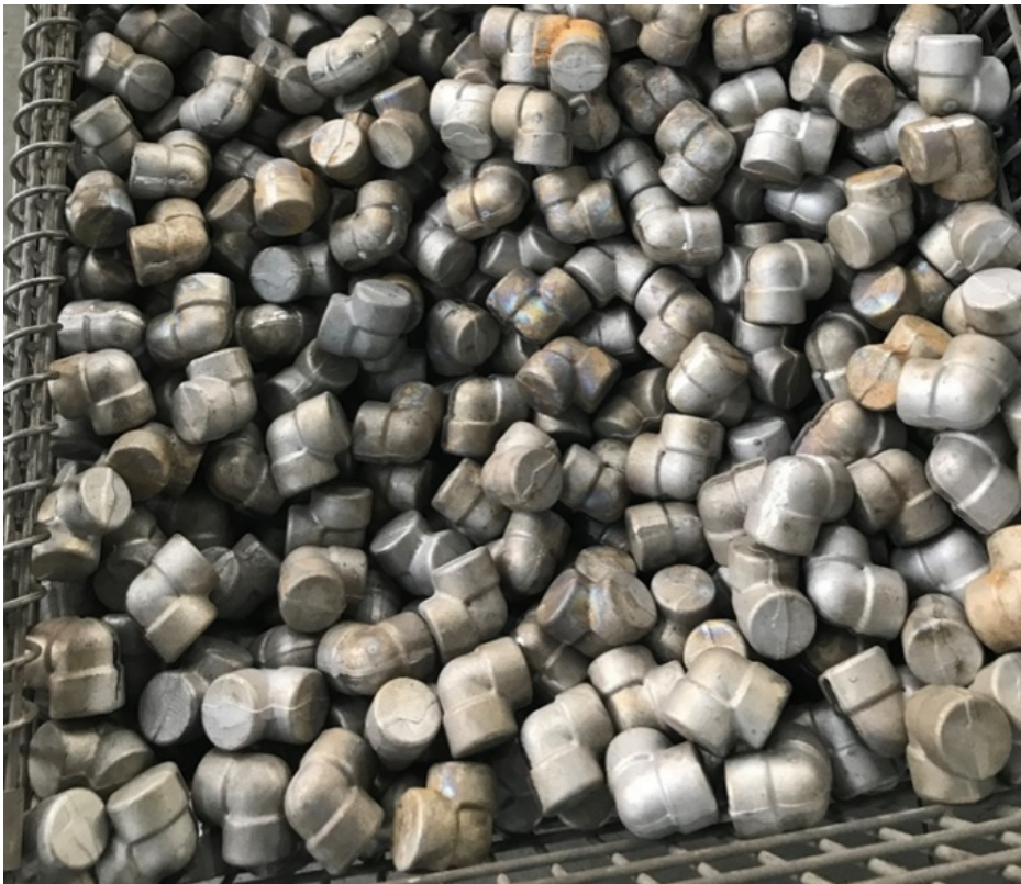
Sand Blast to clean and smooth the surface
